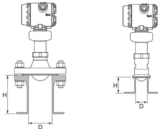
**Table 19: Nozzle Requirements for Process Seal Antenna**
