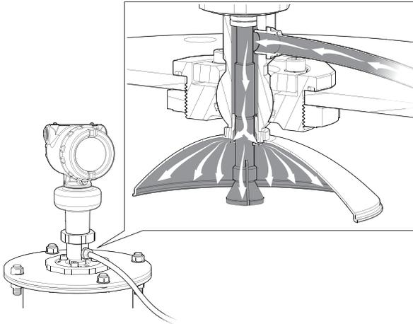
An air purge connection is also available for cone antennas with flanged connection by selecting option code PC1. This option consists of an antenna with purge holes and a separate air purge ring (see [Figure 14](#)).
