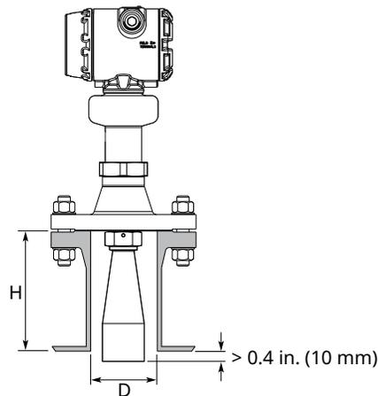
**Table 18: Nozzle Requirements for Cone Antenna, in Inches (Millimeters)**
