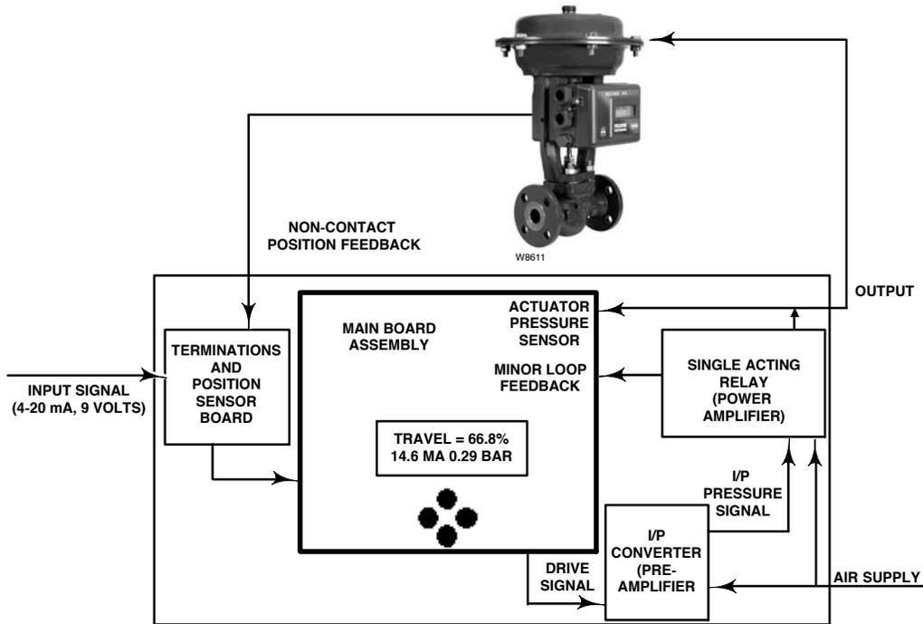
Figure 3. Block Diagram
