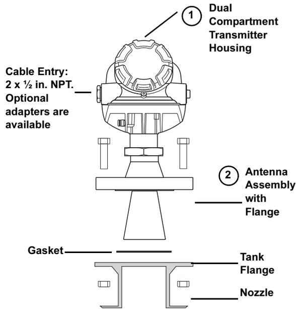
The Rosemount 5400 Series transmitter consists of the transmitter housing and an antenna assembly. The transmitter housing contains all electronics. The antenna assembly seals off the tank atmosphere from the transmitter housing and its surroundings.
