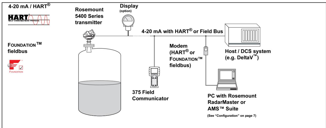
The 5400 Series can be integrated into almost any new or existing plant. Configure it remotely in the control room over the 4-20 mA/Hart® or FOUNDATION™ fieldbus wires. No proprietary connections are needed.
