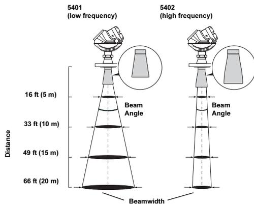
Comparison between the beam angle and beamwidth for the Rosemount 5401 (~6 GHz) and 5402 (~26 GHz) transmitters with antennas of the same size and type.
