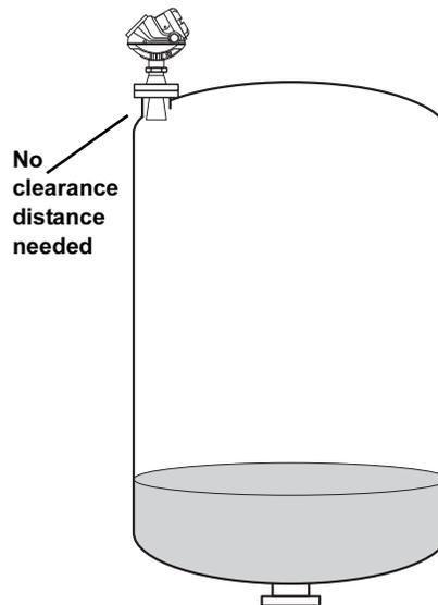
**Circular polarization allows the transmitter to be installed without any clearance distance to the tank wall.**
