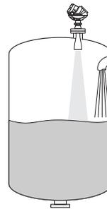
The 5402 transmitter is the preferred choice in most applications because its narrow radar beam offers greater mounting flexibility.
