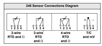
\* Rosemount Inc. provides 4-wire sensors for all single element RTDs. You can use these RTDs in 3-wire configurations by leaving the unneeded leads disconnected and insulated with electrical tape.
