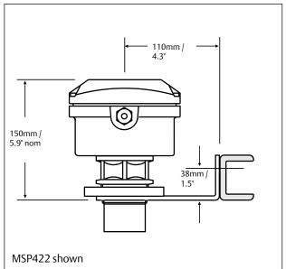
Note: Transmitters are not suitable for mounting in 2" NB pipe. A minimum of 3" NB is required. Use a plastic flange if mounting onto a tank or standpipe.
