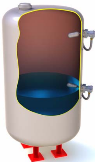
High and Low Alarm Application
