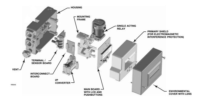
Figure 2. FIELDVUE DVC2000 Digital Valve Controller Assembly (Exploded View)
