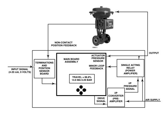
Figure 3. Block Diagram
