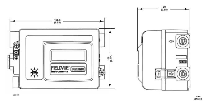
Figure 4. Dimensions for FIELDVUE DVC2000 Digital Valve Controller
