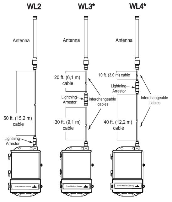
The Remote Omni-Antenna kit includes sealant tape for remote antenna connection, as well as mounting brackets for the antenna, Lightning Arrestor, and the Smart Wireless Gateway.
